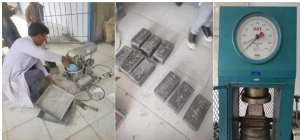
Figure 5: Testing process of compressive strength of paving blocks
